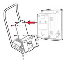
Place Adview on to caddy, carefully aligning the 3 holes on the unit with the 3 holes on the caddy. Using the thumb screws, secure the rear panel of the Adview to the caddy.
