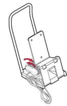
With Power Supply in place, fold over the Velcro® tabs and tightly secure the Power Supply in place.
