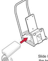
Slide Power Supply between the two Velcro® tabs on rear deck of the caddy.
