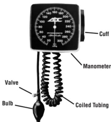
To assemble the inflation system, connect coiled tubing to air inlet nipple at bottom of gauge. Insert male luer adapter on bladder tubing into female receptacle at free end of coiled tubing. Store folded inflation system in swivel bracket behind gauge on 750W and 750D or in integral basket on 752M.
