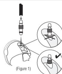
**New 804N Connector:** Insert metal bayonet connector into metal receiver until it clicks (Figure 2).
