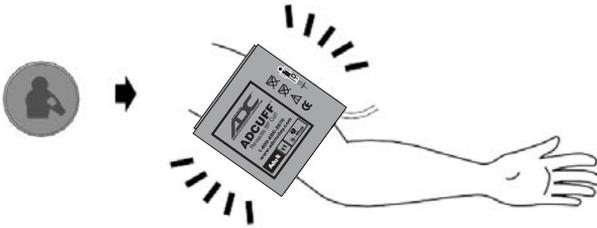
**Re-inflate** – Push and Hold the Memory Button during deflation to re-inflate for as long as the button is held (up to a max of 299 mmHg). Release the button to continue deflation.
