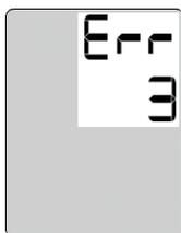
If an error occurs during a measurement, the measurement is interrupted and an error message «Err» is displayed.
