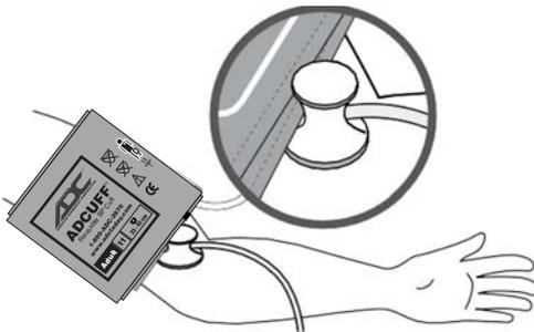
**Start inflation** – Press the Start/Stop Button to begin inflation. When maximum inflation pressure is reached, the e-sphyg 3 will automatically begin linear deflation at a rate of 3 mmHg/sec.
