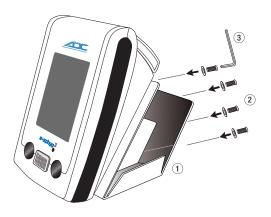
Align the holes on the rear side of the e-sphyg<sup>3</sup> with the four holes on the mounting bracket as shown. Insert the four hex mounting screws and washers through the back of the mounting bracket into the unit and tighten. (Figure 1)
