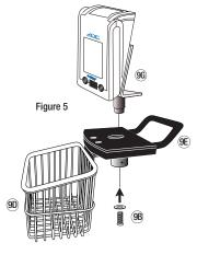
6. Place assembly consisting of the e-sphyg<sup>3</sup>, cuff storage basket and platform on top of stainless steel inner pole, making sure the pole goes completely inside collar. Use tightening device and small hex key as shown.
