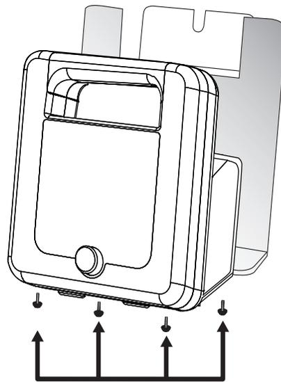
2. Once fully seated, use the hex key to screw in the four mounting screws through the bottom of the caddy into the ADView 2. Hand-tighten all four screws until firmly set.
