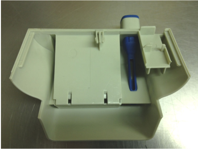
Temperature Probe Well
