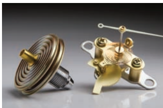
Parts of Aneroid Movement
